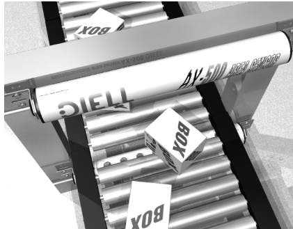
Handling automations: presence detection and object positioning on conveyors
